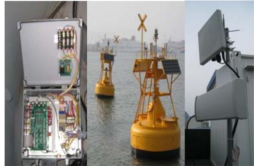
Fig. 9 Experiment system of MPPTS algorithm (Left : MPPTS controller, Middle : buoy, Right : RF-antenna on shore)
