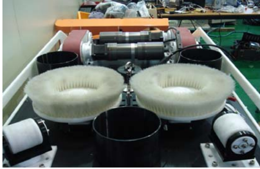
Fig. 3 Down side of the underwater robot with brushes
