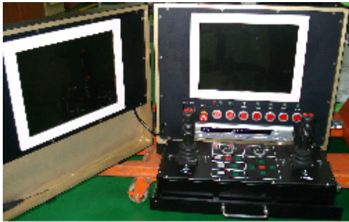
Fig. 6 Photograph of surface control system
