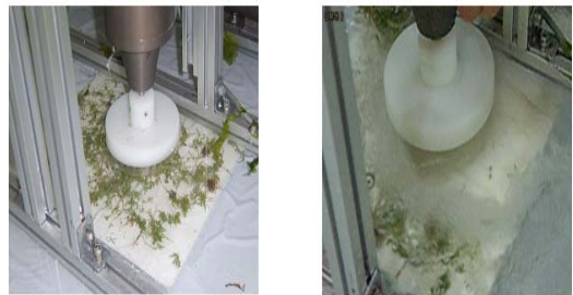
Fig. 15 Cleaning test of the brush system
