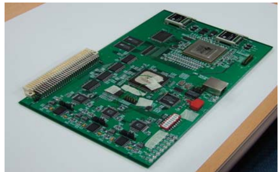
Fig. 9 Servo control board
