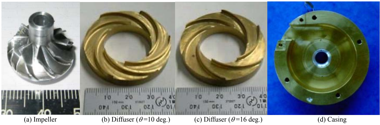
Fig. 3 Tested impeller, diffuser and casing by machining
