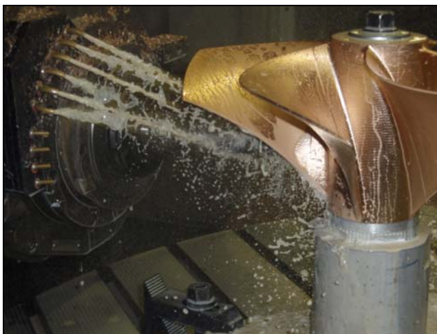
Fig. 20 CNC machining of the model runner
