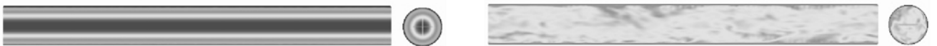
Fig. 1: Instantaneous velocity: initial (left), after 100 cross-flow (right) in the diametral plane and a cross section
