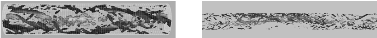
Fig. 3: Visualizations of the flow structure in a periodic swirling pipe flow: L=5D pipe (left), L=10D pipe (right), by the Q criterium
