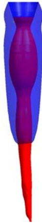
Fig. 10 Comparison of single phase (blue) vs. two phase (red) vortex volume for LC01 in CAD.
