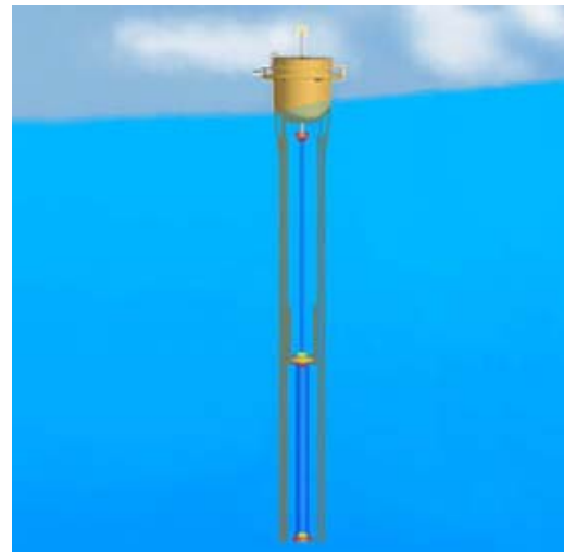
Fig. 5 AquaBuOY Wave Energy Converter [23]
