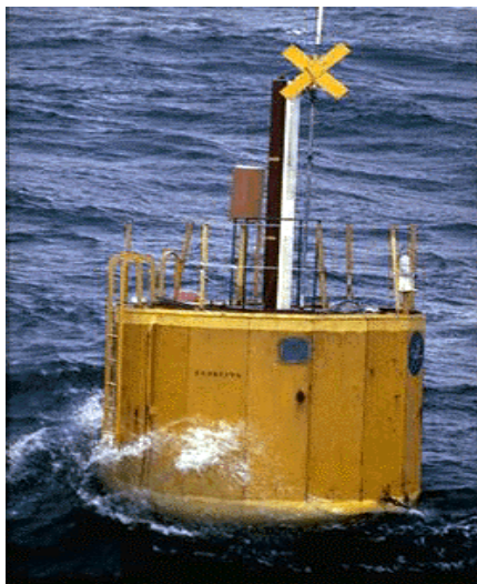
Fig. 4 Point Absorber Energy Converter [22]
