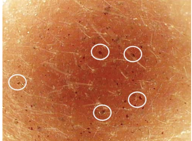
Fig. 2. Optical micrograph of cheek area coated with pearlescent pigment showing small flakes.
