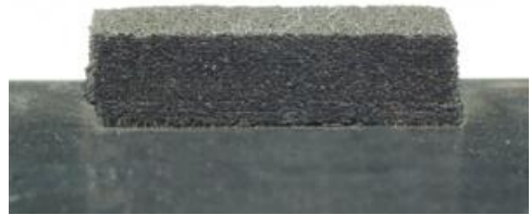
Fig. 6 Laser sintered structure
