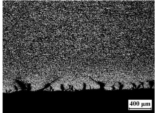
**Fig. 5** Micrographs of the specimen thermally oxidized at 927°C. Surface cracks are initiated at thick  $\alpha$ -case region(gray colored area)
