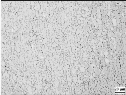
**Fig. 1** Microstructure of Ti-6Al-4V alloy solution heat treated and quenched
