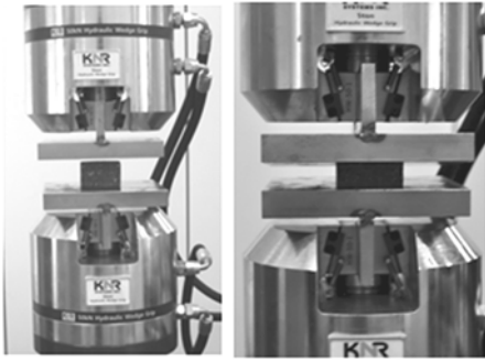
Photo. 3 Quasi-static test of EPP foam
