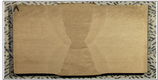
(b) Cross section of EGW welded specimen
