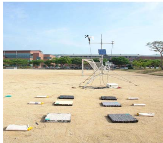
Fig. 1. Field experiment for the estimation of latent heat flux on the water retention pavement materials. The pole indicates the Automatic Weather System including several meteorological equipments.
