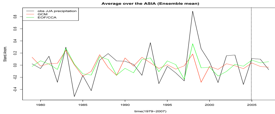
Figure 4.1. Time series of the comparing prediction for the Asia precipitation. The observed precipitation (black line), GCM output (red line), and the result of the hybrid method (green line) are displayed.
