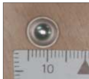
Fig. 1. The titanium cap (annealed, 99.5%, Johnson Matthey Company, USA) had a height of 4 mm, diameter of 8 mm, and thickness of 0.25 mm.
