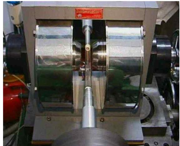
Fig. 3 Photo. of experimental equipments for magnetic abrasive polishing
