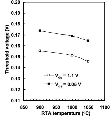
**Fig. 8.** Variation of threshold voltage with RTA temperature.
