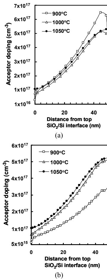
**Fig. 5.** Acceptor doping profile from top Si/SiO<sub>2</sub> interface to bottom Si/BOX interface at various RTA temperature (a) at the middle of the gate, (b) 0.5 nm away from the sidewall Si/SiO<sub>2</sub> interface. The corresponding cut-lines were drawn at a vertical plane equidistant from source and drain.
