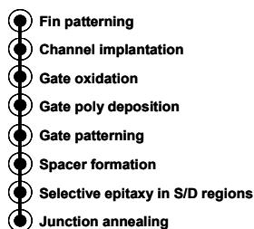
**Fig. 2.** Simulated process flow for FinFET devices.
