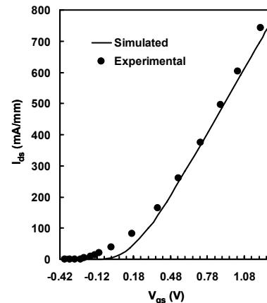
**Fig. 3.** Calibrated transfer characteristics at drain to source voltage of 1.2 V.
