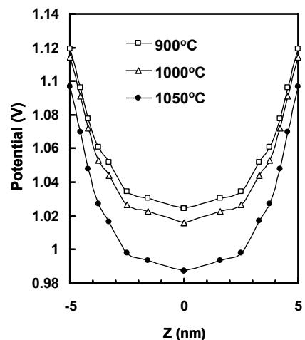
Fig. 7. Potential variation between two vertical Si/SiO<sub>2</sub> interfaces of TG-FinFET at various RTA temperatures. The corresponding cut-lines were drawn 1 nm below the top Si/SiO<sub>2</sub> interface in a cut-plane equidistant from the source and drain.  $V_{gs}$  and  $V_{ds}$  are kept at 1.0 and 1.1 V respectively.
