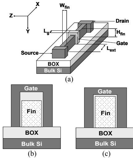
**Fig. 1.** (a) Schematic of a triple gate FinFET. 2-D cut plane view of (b) DG FinFET and (c) TG FinFET.
