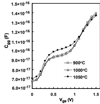
**Fig. 9.** Variation of total gate capacitance ( $C_{gg}$ ) with gate to source voltage ( $V_{gs}$ ) at different RTA temperatures. The drain to source voltage is kept at 1.1 volt.
