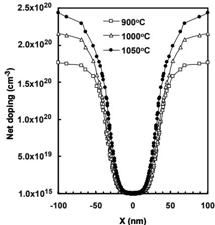
**Fig. 4.** Net doping profiles along channel at various RTA temperatures. The corresponding cut-lines were drawn 1 nm below the top Si/SiO<sub>2</sub> interface for all the devices.
