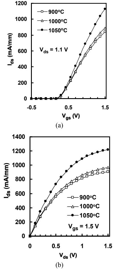
Fig. 6. (a) Transfer characteristics and (b) output characteristics are shown as a function of RTA temperatures.
