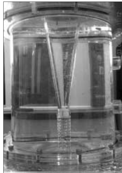
Fig. 8. Structure of HCF-closed system with underflow screen.
