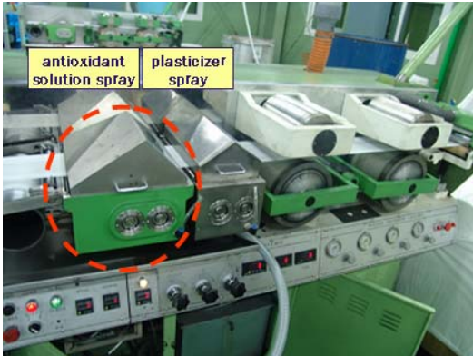
Fig. 4. Apparatus of brush type atomizer for antioxidant application to filter.
