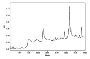
**Fig. 5.** HPLC Chromatogram of the SSE. The solution of SSE was prepared by dissolving in distilled water (10 mg/100 ml). The injection volume was 20 ml and the detection was made at 254 nm.
