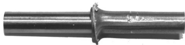
Fig. 7 Appearances of friction weld specimens of Vit-1/A5083 (at P_f=150 MPa, t_f=0.6 s)
