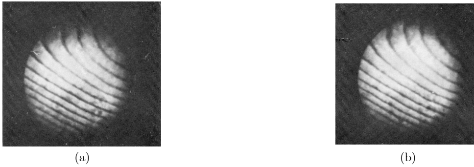
FIG. 4. Two digital interferograms after high spatial frequency removal : (a) when phase step \varphi_i = 0 , (b) when phase step \varphi_i = \pi/2 .
