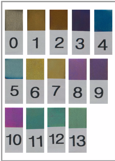
Fig. 2. Photographs of titanium specimens fabricated by anodization.
