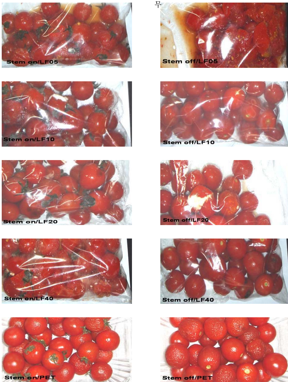
Fig. 7. Photograph of stem on/off cherry tomatoes, after storage of 20days in PET container, LF05, LF10, LF20, and LF40 film packaging.
