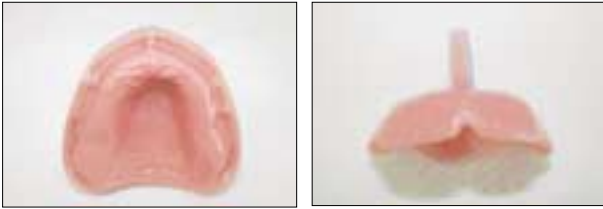
Fig. 1. Dentiform and denture base used to test tensile bond strength of denture adhesive.
