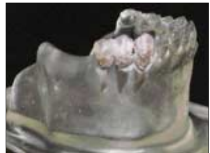
Fig. 3. Photoelastic model with the duplicated resin teeth.
