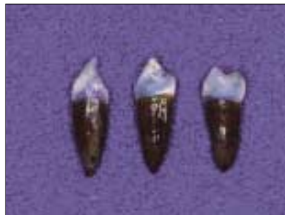
Fig. 2. Duplicated resin teeth with the simulated periodontal ligament.
