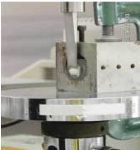
Fig. 4. Shear bond strength test in Universal testing machine.
