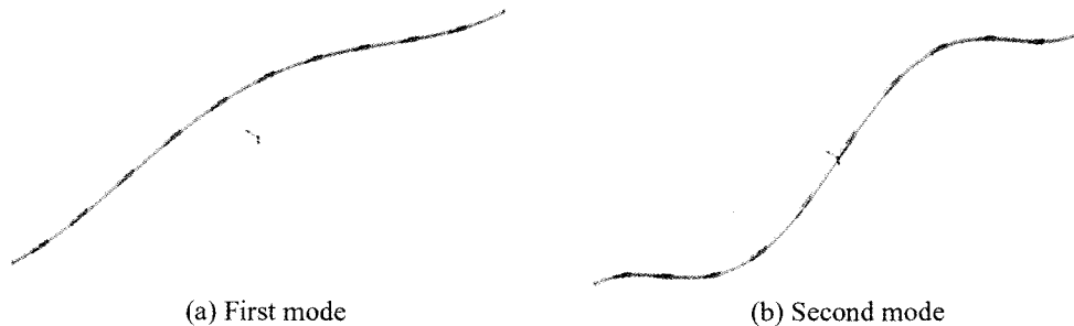
Fig. 8. The First Two Modes in a 3-D Model
