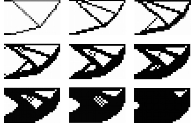
Figure 5. Topology with respect to different volume fractions ( V_f ): (a) 10%, (b) 20%, (c) 30%, (d) 40%, (e) 50%, (f) 60%, (g) 70%, (h) 80% and (i) 90% of the volume of the initial configuration of the beam
