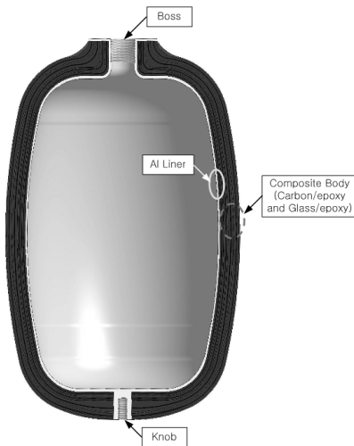
Fig. 1. FEM analysis model of aluminum-carbon/epoxy-glass/epoxy composite tank.
