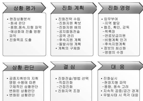
Figure 4. Flowchart of helicopter suppression on forest fire.
