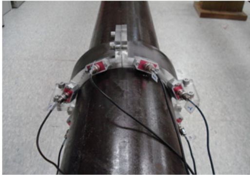
Fig. 7 Experimental setup for array guide waves testing for a pipe
