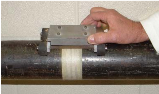
Fig. 1 DC bias magnetization of magnetostrictive strip by a permanent magnet
