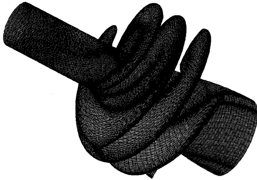
Fig. 5 Computational grid for 3-bladed inducer (3 blocks, 277,551 cells)
