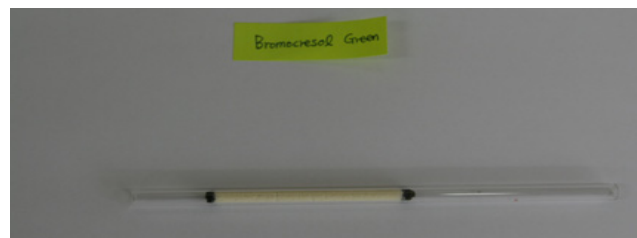
Fig. 2. Detector tube for ammonia measurement.
