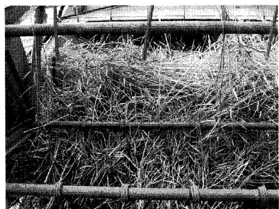
Fig. 6 Problem of stem and pod obstruction in rapeseed harvesting.
