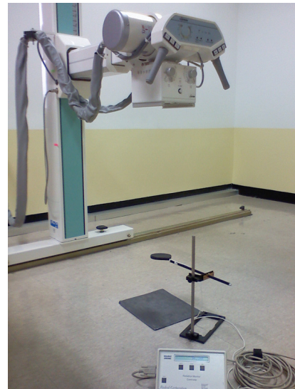
Fig. 1. Arrangement diagram to measure the output x-ray dose
