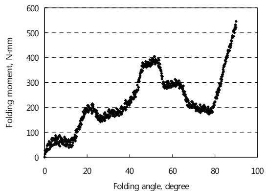
Fig. 7. Folding moment behavior of A flute corrugated fiberboard with score.
