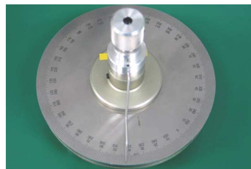
Fig. 2. A device for measuring the amount of rotation.
