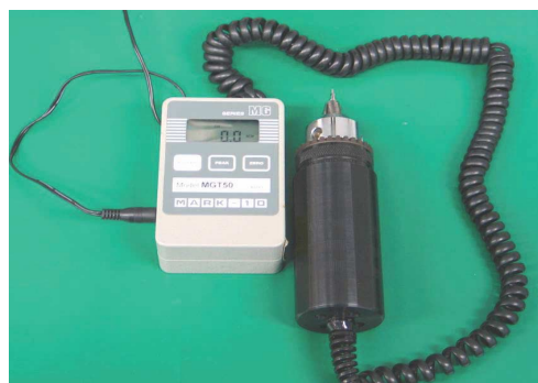
Fig. 3. The digital torque gauge used in current study.
