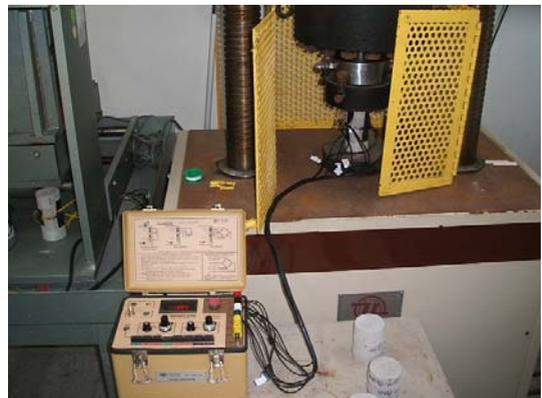
**Fig. 3 Measurement of uniaxial compression strength and poisson's ratio**
