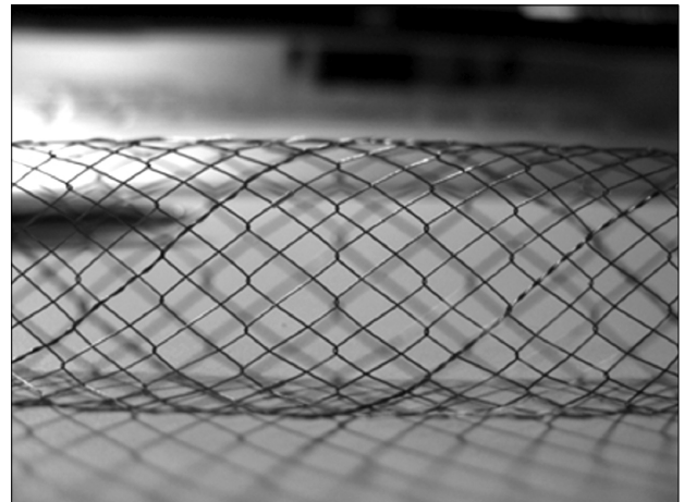
Fig. 2. Design and construction type of stent.
