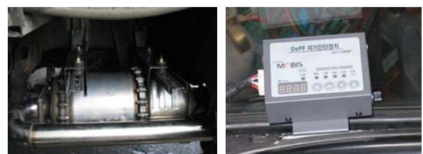
Fig. 2 Configuration of vehicle data monitoring system
