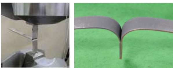
(a) T-peel test (b) Failure mode of specimen Fig. 14 Cohesive mode of T-peel specimen
