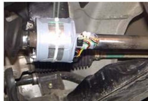
Fig. 6 Strain gages and telemetry system
