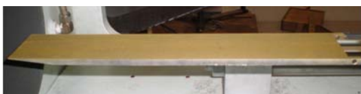
Fig. 4. Long plate model for detection of boundary layer transition
