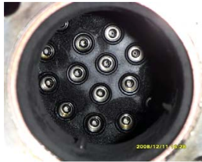
Fig. 17. Gas generator faceplate after 595 sec firing tests
