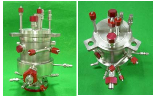
Fig. 9. 30-tonf LRE gas generator
