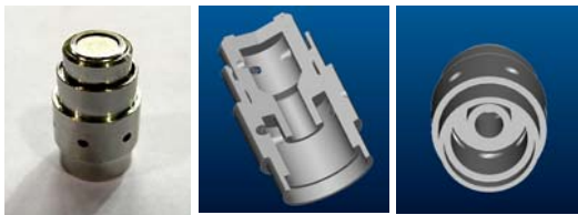
Fig. 2. Photographic view of the Injector (left) and its 3D modelling works
