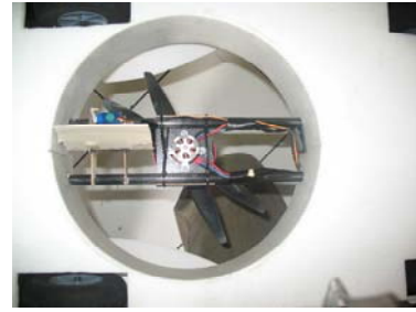
Fig. 10. Yaw control of ITB unmanned PAV prototype
