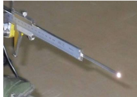
Fig. 9. A vernier caliper with reflective paper attached for parallel direction test
