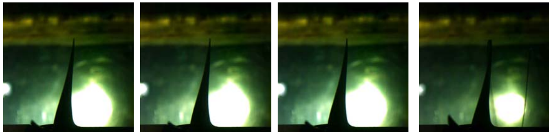
(a) 0 N 25 rps (b) 250 N 25 rps (c) 500 N 25 rps (d) 750 N 25 rps Fig. 4 Blade image of flexible propeller with thrust variation in uniform flow(upper part) (Hyun et al. 2008)
