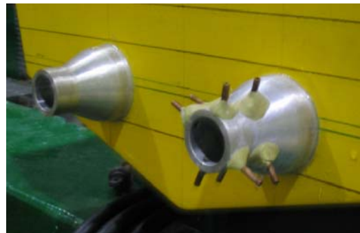
Fig. 6 Profile of waterjet nozzle and pressure tabs
