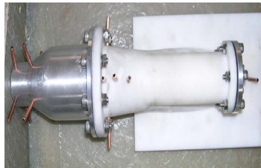
Fig. 3 Waterjet model with pressure tabs
