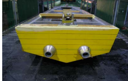
Fig. 2 Profile of model ship equipped with waterjet system
